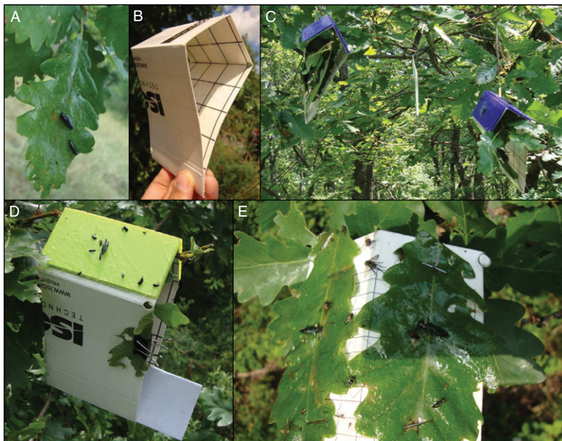
Figure 1 Trapping designs that were employed both with and without visual decoys, including (A) sticky leaves, (B) a white branch-trap, (C) purple plastic branch-traps with a ( Z )-3-hexen-1-ol packet suspended between them, (D) a green plastic branch-trap with a ( Z )-9-tricosene packet attached to the underside, and (E) a leaf-covered branch-trap.
