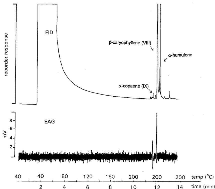
FIG. 5. Reconstructed simultaneously recorded gas chromatogram [flame ionization detector (FID)] of a mixture of  $\alpha$ -copaene,  $\beta$ -caryophyllene, and  $\alpha$ -humulene (top) and electroantennogram (EAG) of a female medfly antenna (bottom). EAG active compounds are labeled VIII and IX (see text for details).
