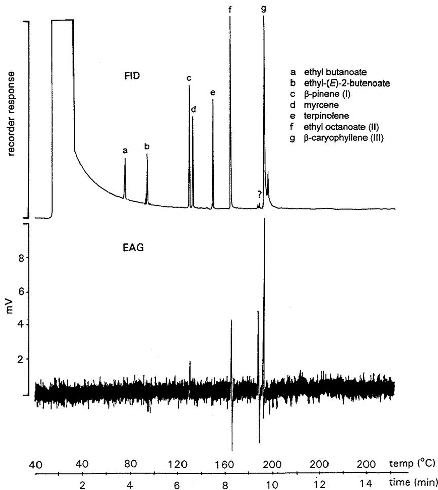
FIG. 4. Reconstructed simultaneously recorded gas chromatogram [flame ionization detector (FID)] of a mixture of commercial and synthetic compounds identified from ripe mango (top) and electroantennogram (EAG) of a female medfly antenna (bottom). EAG active compounds are labeled VI, VII, VIII, and ? (see text for details).
