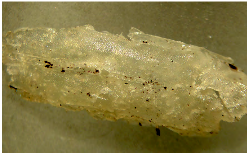
Figure 6. Photograph of a partial decoy made of PET.
