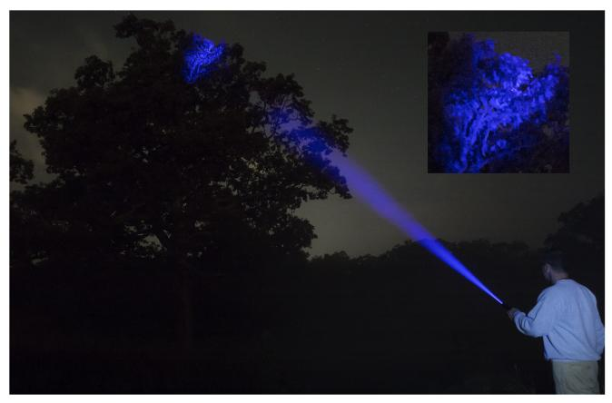
Fig 2. A fluorescent-marked brown marmorated stink bug detected using handheld laser equipped with a focusing lens. The oak tree in the picture is 27-m high. The specially designed goggles that we used eliminated the purple light of the laser (seen blue in the picture) and transmitted, with no interference, the light from the glowing, marked insect. The inset shows the marked insect (in red), which is clearly visible to the laser operator.
