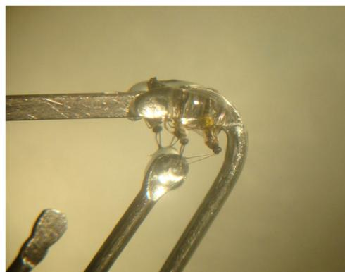
**Fig. 2** Close-up image of the setup used for GC/EAD recordings. Four *Lycoriella ingenua* males' abdomens formed an electrical connection with one of the stainless steel electrodes on the Quadroprobe using electroconductive gel, and their eight antennae contacted the second, recording electrode such that the eight antennae were placed in parallel
