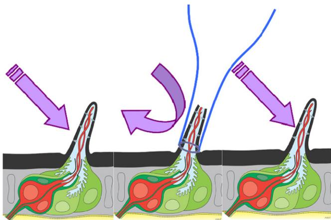
Fig. 3. Schematic diagram illustrating the method for covering a sensillum with the recording electrode and the presentation of the pheromone odorant. Complete covering prevents the sensillum from being exposed to the airborne stimulant while the neighboring sensilla are exposed. The illustration was modified from Steinbrecht (1999).
