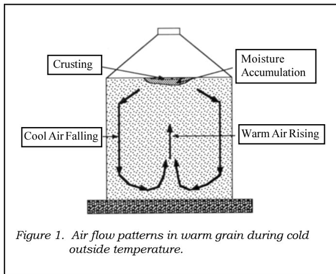
Figure 1. Air flow patterns in warm grain during cold outside temperature.
