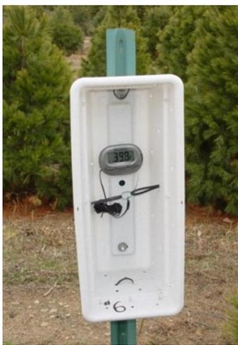
Max/Min Thermometer station [PDA]
