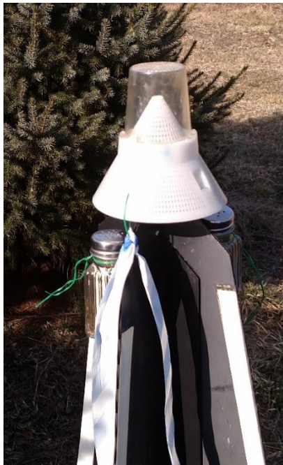
Top of white pine weevil trap baited with ethanol and turpentine. [S. Pickel, PDA]
